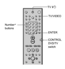
Press and hold TV I/(1) while entering your TV's manufacturer's code (see the table) using the number buttons and press ENTER. Then release TV I/(1).
